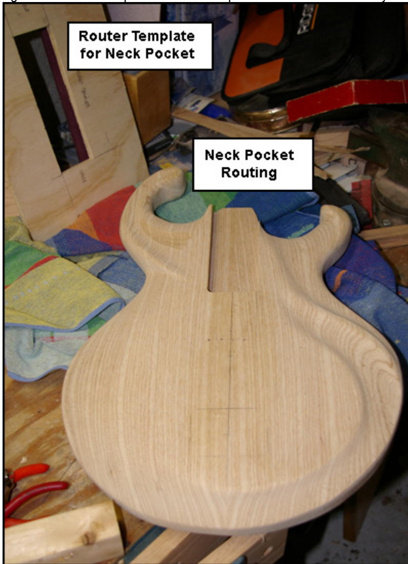
Figure 19 A router template and the neck pocket routed out of the body
