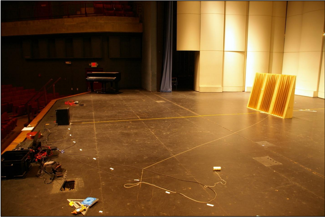
Figure 35 Full view of vertical testing showing the test speaker and the diffuser being tested.
