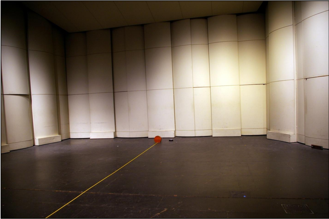
Figure 26 The stage is bisected with a landscaping tape and held in place with an Earthworks microphone case. This is the initial measurement from which the testing radius is created.
