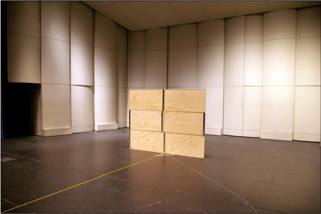
Figure 33 A Flat Panel array in testing position was created simply by reversing the diffusers under test and exposing the flat backs. The flat mounting bands of darker color and the slight differences in angle of the panels may have caused errors in the data collection.
