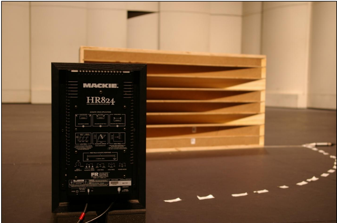
Figure 45 Testing the Acoustic Ramp in horizontal position in the 5' radius testing setup.
