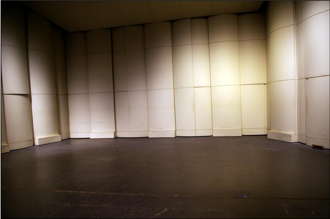
Figure 25 University of Massachusetts Lowell's Concert Hall stage with the shell installed. This is the largest available space for acoustic testing in the Music Department's Durgin Hall. From center down stage nearly 25 feet of testing distance is available before the first reflection point.
