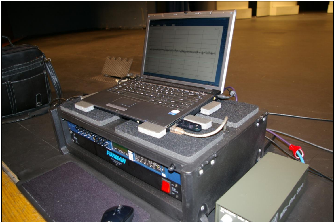
Figure 40 Testing hardware system. Windows XP laptop using ARTA acoustic testing software, a MOTU Traveler, and a Daking Audio Mic Pre One.
